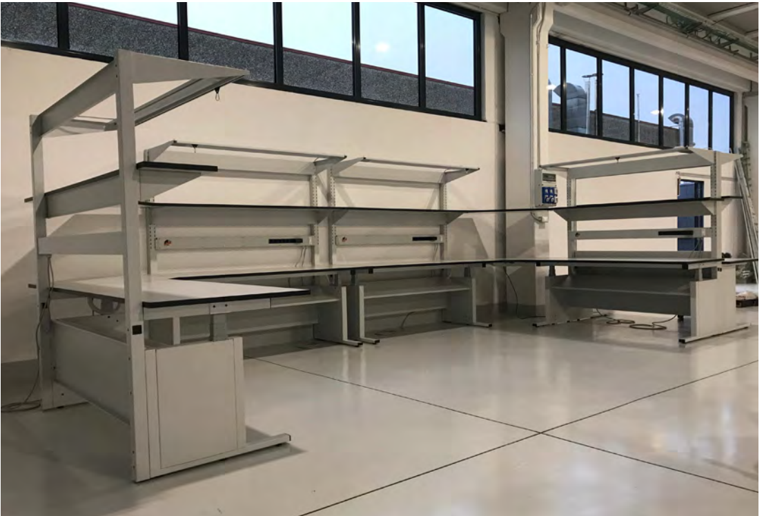
It's possible to millimetrically adjust the entire configuration thanks to the button control panel mounted under the worktop.
