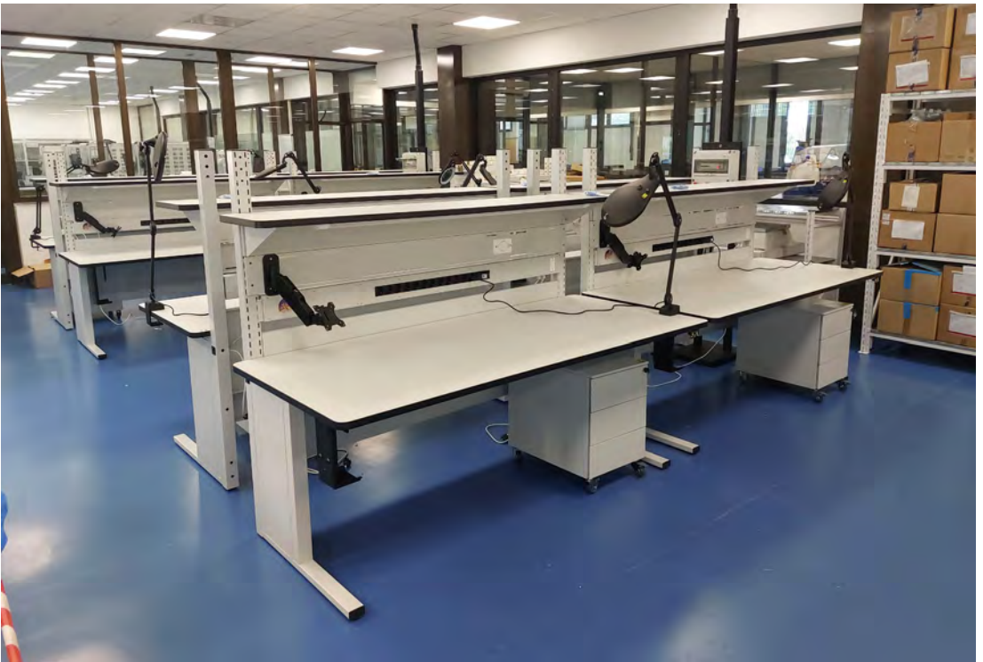
KE MEDIUM workbench with monitor holding arm and bar, ESD-SAFE lens and chest of drawers.
