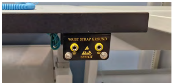
Grounding node (pg.148) fitted under the workbench
