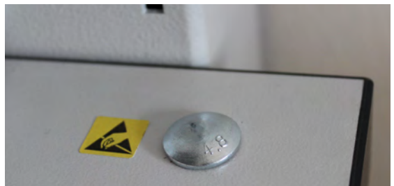
Grounding node (pg.148) fitted under the workbench
