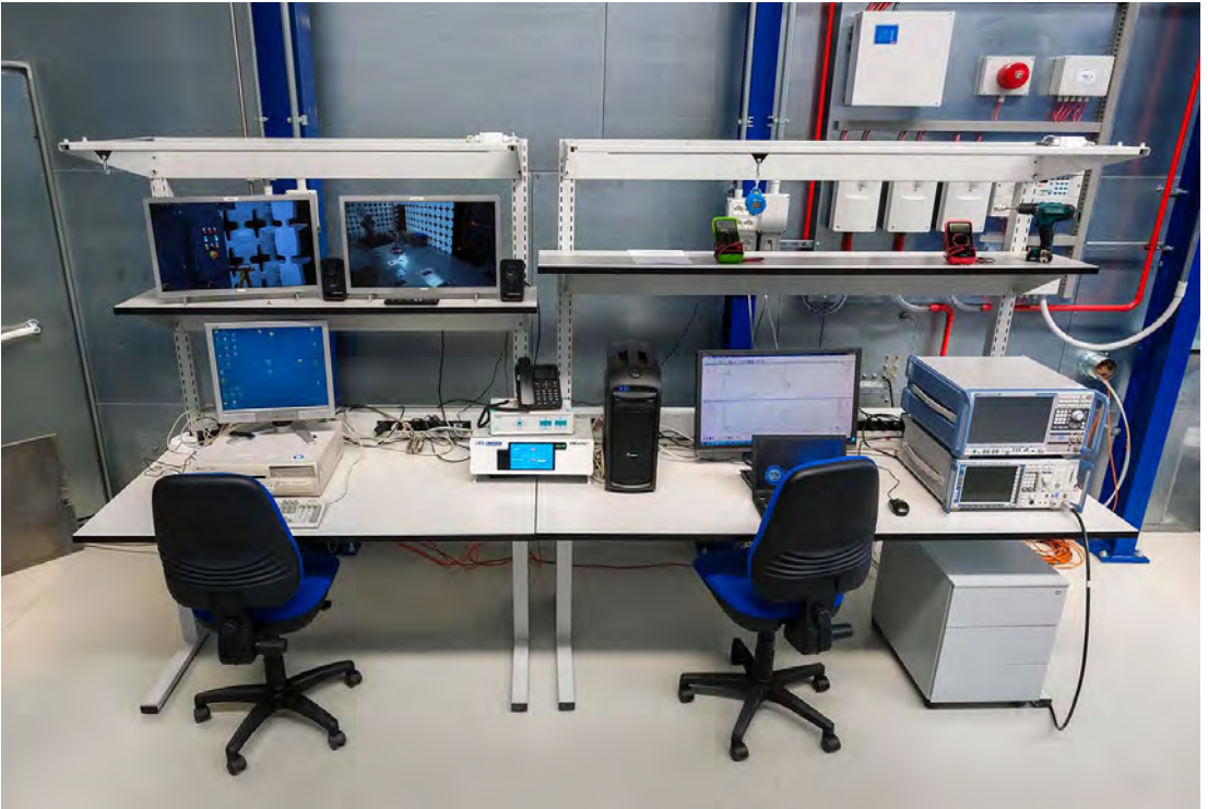
KE HIGH ESD-SAFE workbench for electromagnetic compatibility.
